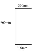
Q.18 The stiffened cross-section of a long slender uniform structural member is idealized as shown in the figure below. The lumped areas at A, B, C and D have equal cross-sectional area of 3 cm<sup>2</sup>. The webs AB, BC, CD and DA are each 5 mm thick. The structural member is subjected to a twisting moment of 10 kNm. The magnitudes of the shear flow in the webs,  $q_{AB}$ ,  $q_{BC}$ ,  $q_{CD}$ , and  $q_{DA}$  in kN/m are, respectively
