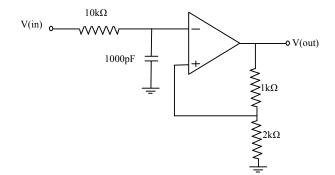
Q.54 For this circuit the frequency above which the gain will decrease by 20 dB per decade is
