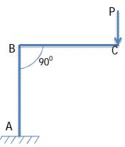
Q.17 Neglecting the axial compression of member AB, the deflection of point C in the direction of the load is
