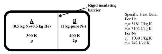
Initially, chamber A contains a mixture of 0.5 kg nitrogen and 0.5 kg helium at 300 K while chamber B contains 1 kg of pure nitrogen at 400 K. The pressure in chamber B is twice that in chamber A. The gases and gas mixtures are assumed to be ideal.
