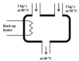
There is no accumulation of water in the tank. A back-up heater is provided to ensure a constant outflow temperature of water at 60  $^{\circ}$ C from the tank under steady state. What is the required capacity of the back-up heater to the nearest kW?
