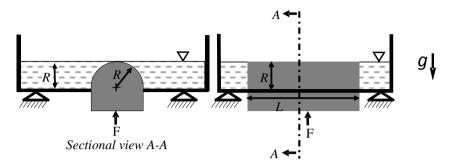
The force F required to hold the plug in its position is
