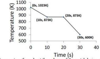
Assuming uniform temperature throughout the volume of the metal during solidification, the latent heat of fusion of the metal (in kJ/kg) is \_\_\_\_\_
